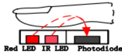
Fig. 1. Reflective type oxygen saturation detection [2]
