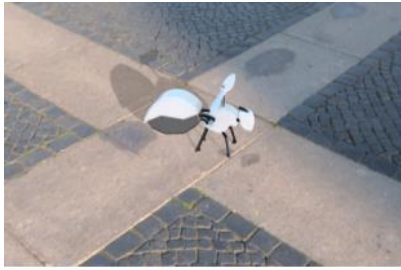
Figure 2: Robo-bee compared to floor tiles (rendered image Auto-desk fusion 360)
