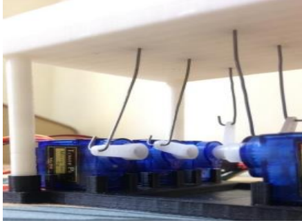
Fig. 4 Dot raising mechanism
